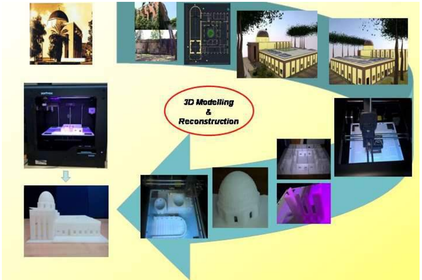
Figure 3.10. Design of a physical model of the building (Chiesa di Santa Maria Francesca Saverio Cabrini – ex Padiglione della Civiltà Cristiana in Africa, Mostra d'Oltremare – Naples, Italy) integrating image capture and analysis techniques with FDM.
